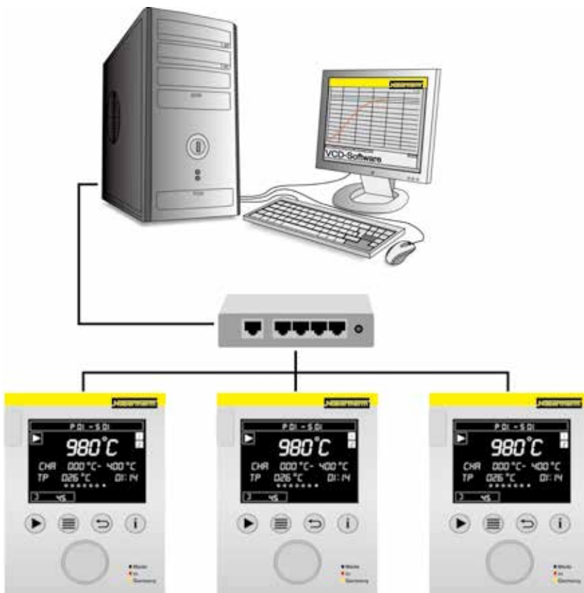
Example lay-out with 3 furnaces
